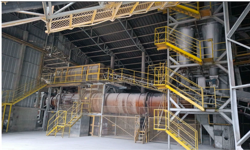
Figure 6: Rotary Drying and Cyclone System
