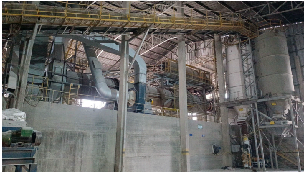
Figure 7: Silo System, Dryer and Gas Scrubber
