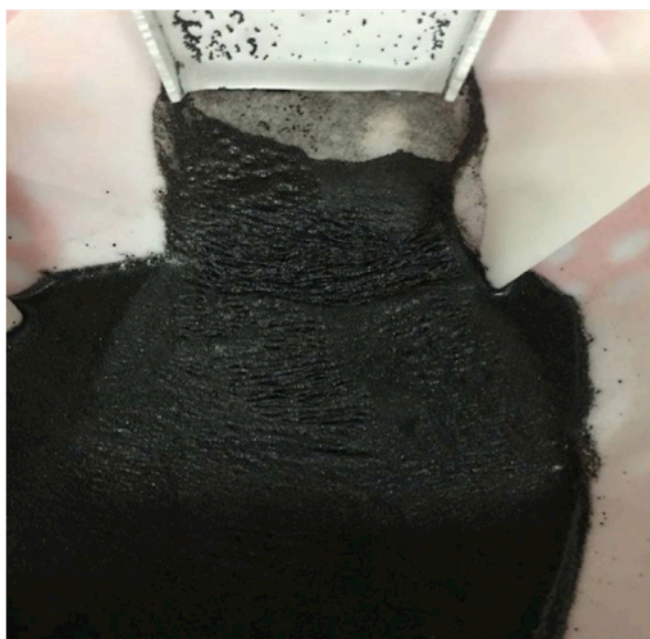
Diagram 2: Initial graphene recovery from 2.5 litre cells at University of Adelaide (April. 2016)
